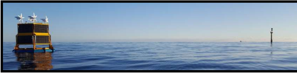
Figura 4 - Floating LiDAR System instalado na bóia RPS Lidar 4.5 Buoy (RPS, 2021).
